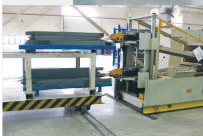
▲ ③ Automatically stacked silicon steel sheets
