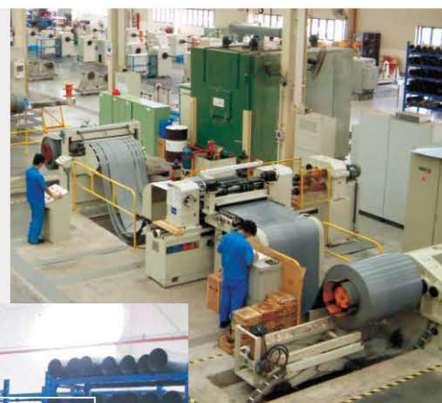
▲ Cutting line (Slitting)
